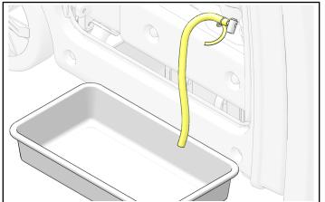
4. Loosen the carburetor drain screw and drain the fuel.
