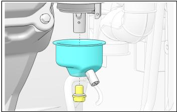
9. Remove the main jet from the carburetor.
