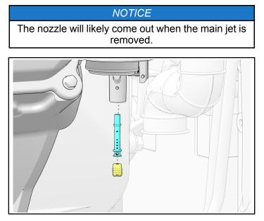
10. Install the correct main jet for the altitude in which the generator is operating. Do not over-tighten the jet.
