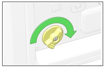
2. Loosen the two maintenance cover fasteners and remove the cover.
