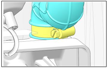
7. Remove the two fasteners securing the air filter box and remove the box.
