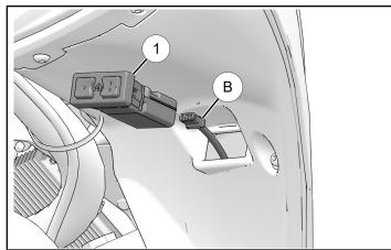
5. Insert Garage Door Opener ① into hole. Apply pressure until module clicks into place.
