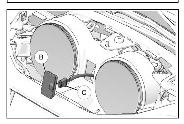
5. Locate harness connection on back of Garage Door Opener ①. Click wire harness branch ⓒ into module.
