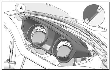
2. Apply pressure to top of gauge hood until hood snaps into place.
