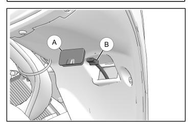
4. Locate harness connection on back of Garage Door Opener ①. Click wire harness branch ® into module.
