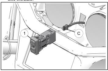
6. Insert Garage Door Opener ① into hole. Apply pressure until module clicks into place.
