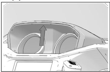
2. Apply force until gauge hood (A) pops off dash support. Remove gauge hood.
