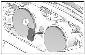
4. Grasp both grommet ® and wire harness branch ©. Disconnect grommet from harness. Discard grommet.
