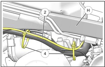
9. Route wiring 2 behind frame (1) and secure to existing harness (K) with new cable tie (4). Continue to route wire (2) behind fork (1) toward headlight housing.
