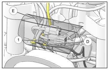
2. Reinstall headlight nacelle and brackets with six retained screws. Torque screws to specification.
