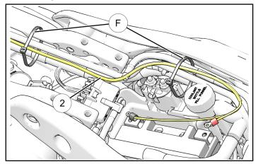
5. Connect positive (+) battery cable C and positive end of new USB wire 2. Secure using retained screw (E). Torque screw to specification.
