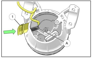
Plug speedometer connector into speedometer. Ensure USB wiring is routed properly and reinstall speedometer mount assembly <sup>(B)</sup> using four retained bolts <sup>(C)</sup> (removed in Step 1 of Speedometer Mount Removal section.) Torque bolts to specification.
