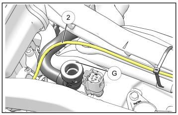
8. Route wiring (2) under upper frame (#). Secure wire to main harness with cable tie (4).
