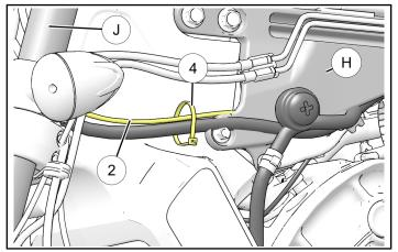
10. Insert wire end (2) into opening on rear of headlight housing (K) and pull through opening into headlight housing.
