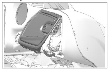
4. Secure each grill with two screws in bottom edge of each fairing speaker grill. Torque screws to specification.
