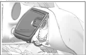
4. Remove and retain two screws (A) from lower portion of inner fairing, and four screws (B) and washers (C) from middle outside of inner fairing.
