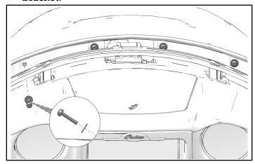
2. Remove and retain two screws from bottom edge of each fairing speaker grill.
