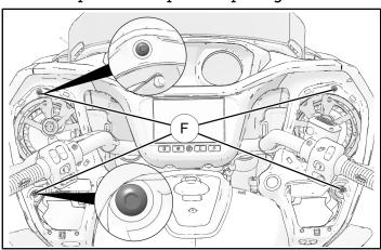
6. Remove and retain one screw © from under edge of each side of fairing as shown.
