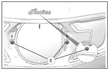
7. Torque all outer fairing screws to specification.
