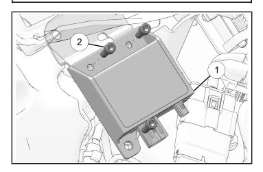
3. Locate both connectors (B) and (C), cut retaining zip-ties (if needed for length) and connect to module (1).
