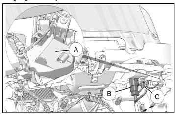
2. Unplug connectors (B) and (C) and bring to module. Cut retaining zip-ties (if needed for length). Set module (1) in place under tab and secure with push-pin rivot (3).
