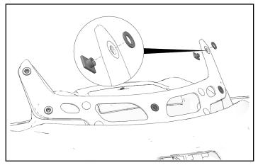
3. Set windshield in place and secure with five screws. Torque screws to specification.
