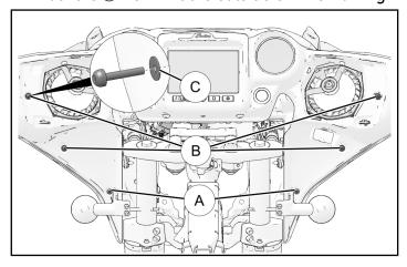
5. Carefully remove outer fairing and set aside on a non-scratch surface.
