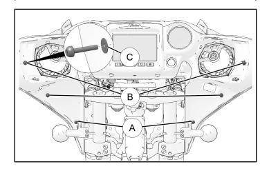
3. Rotate speaker grill from top and install into fairing.
