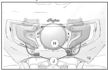
3. Press fairing into place and at top edge to engage locating pins.
