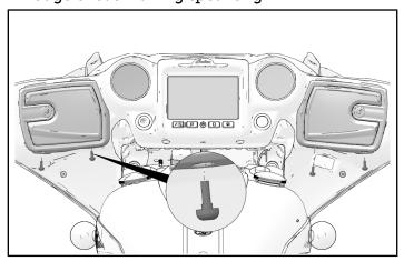
3. Rotate speaker grill from bottom and remove from fairing. Carefully set aside on a non-scratch surface.
