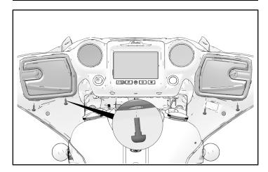
5. Install four screws to top edge of fairing, directly below front edge of windshield bracket. Torque screws to specification.
