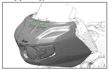
4. Loosely install one screw (6) into hole under edge of each side of fairing as shown. **DO NOT** torque fastener at this time.
