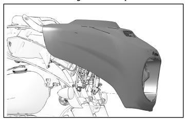
2. Secure with two screws (A) in lower portion of inner fairing, and four screws (B) and washers (C) in middle outside of inner fairing. Torque screws to specification.
