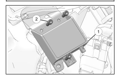
3. Locate both connectors (B) and (C), cut retaining zip-ties (if needed for length) and connect to module (1).
