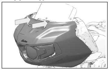
4. Loosely install one screw © into hole under edge of each side of fairing as shown. **DO NOT** torque fastener at this time.
