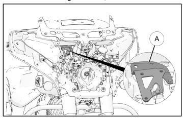
2. Set module ① in place and secure with three new screws ②. Torque screws to specification.
