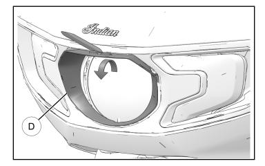
4. Remove and retain three screws © from around headlight bezel as shown.
