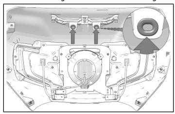
2. Set outer fairing in place and connect turn signal  $\bigcirc$  and headlight  $\bigcirc$  wire connectors.
