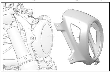
2. Install headlight cowl with retained washers and fasteners.
