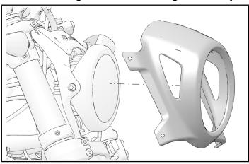
2. Install headlight cowl with four washers 6 and four fasteners 5.
