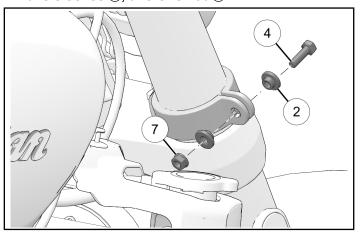
2. Rotate cowl mount on fork and hand tighten fastener.
