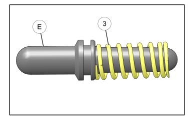
3. Install new boot ④ onto push-rod/spring assembly (E) as shown (Spring is installed *inside* boot). Ensure boot is seated into gap on push-rod.
