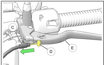
Remove and discard pivot cap €, pivot bolt €, and nut ⊕ from clutch lever €.
