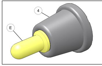
4. Install push-rod/spring/boot assembly (E) into master cylinder body (G). Lightly press edges of boot into body with slotted screwdriver to fully seat boot.
