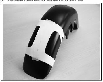
7. Ensure template is centered on fender using a flexible ruler. Measure from centerline to fender edge. Distances should be identical from side to side. Measure in a few locations along centerline to verify template is installed properly.
