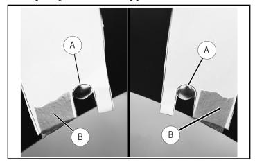
5. Align edges of template with edges of fender as shown and secure with masking tape <sup>®</sup>. Template will pivot on hinges slightly.
