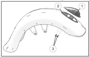
2. Ensure headdress is centered and straight. Torque screws to specification.
