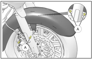
2. Stand in front of motorcycle facing front fender and squeeze sides together while "rolling" fender out from fork legs.
