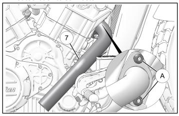
4. Slide clamp ® onto rear header ④ with nut facing down and outward as shown. Insert front header pipe into rear header pipe opening and slide rear header into place. Loosely install rear exhaust header using two retained nuts ⑥. Ensure Oxygen Sensor wiring is routed back to connector.
