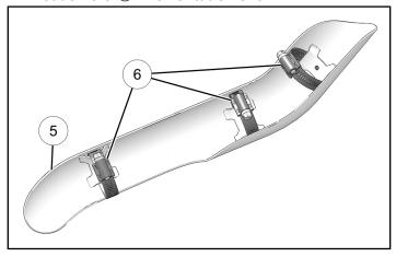
4. Install lower front heat shield (5) in place and secure with three clamps (6). Torque clamps to specification.
