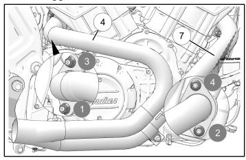
6. Torque exhaust header nuts to specification in same order as previous step.
