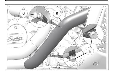
5. Install rear heat shield ① to secondary pipe, install Loctite® onto threads of two screws ① and secure heat shield with two screws ①. Torque screws to specification.
