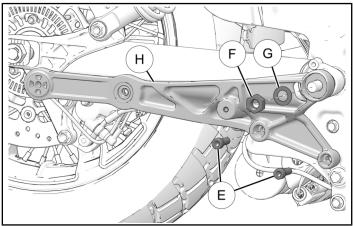
5. Remove and retain two washers ①, four rubber grommets ® and two sleeve washers ① from stock muffler mount ®.
