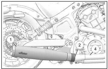
3. Align muffler assembly, rotate muffler clamp ② away from ground and torque clamp ② and mounting bracket screws ③specifications.
