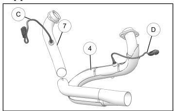
2. Install new exhaust header gaskets 4.
