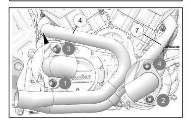
7. Torque Oxygen Sensors to specification.
