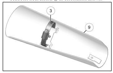
2. Install collector heat shield (9) by first inserting tab (shown with inset) under rear edge of installed heat shield, then securing with clamp
