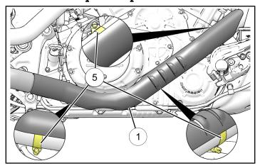
3. Ensure seam between front ① and rear lower ③ heat shield is even and shields are straight. Tighten hose clamps to specification.
