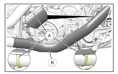
2. Cut two small clamps © and one larger clamp ® and remove rear lower heat shield.
