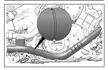
4. Open clamps far enough to slip them over exhaust pipe and install rear upper heat shield
