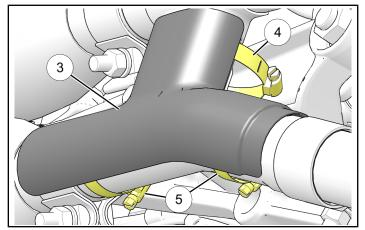
2. Open clamps far enough to slip them over exhaust pipe and install front heat shield ① over exhaust pipe. Loosely install hose clamps ⑤. **DO NOT torque clamps at this time.**
