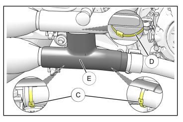
3. Cut three clamps (f) and remove rear upper heat shield (G).
