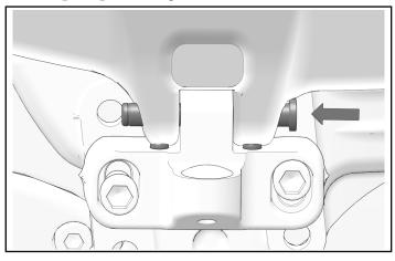
3. Secure pin with retaining ring.
