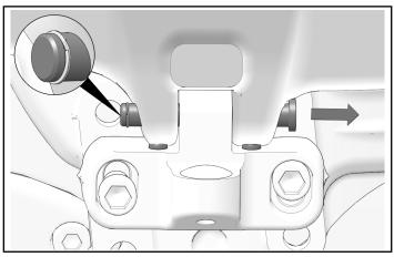
3. Make note of detent balls and compression springs.
