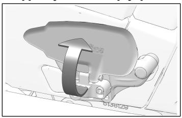
2. Remove retaining ring and slide pivot pin out to remove floorboard from mount.
