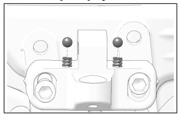
2. Align accessory floorboard with pivot mount and pass pin through floorboard and mount.
