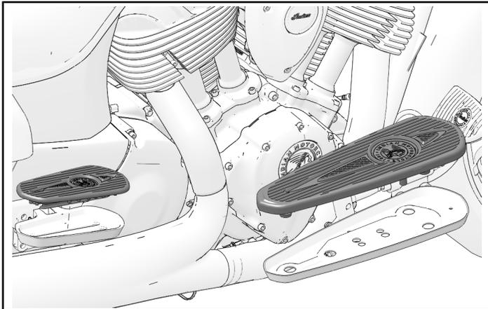
2. Ensure rubber protrusions are fully engaged with floorboard frame as shown.
