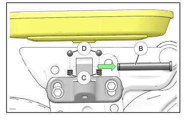
5. Ensure two Detent Springs © and two Detent Balls <sup>(B)</sup> are installed in Floorboard Mount holes.
