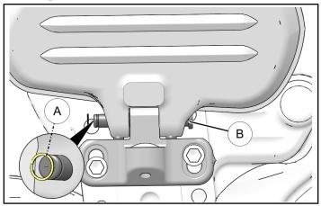
b. Remove pin (B) by pressing out towards large end. Use caution not to lose Detent Balls (D) and Detent Springs (C) when removing original floorboard.
