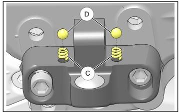
6. Carefully place Floorboard ① into position, depressing springs and balls into pivot. Align holes and insert pin (A) from front side.
