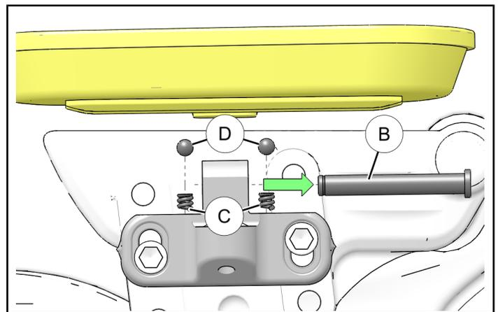
5. Ensure two Detent Springs **C** and two Detent Balls **D** are installed in Floorboard Mount holes.
