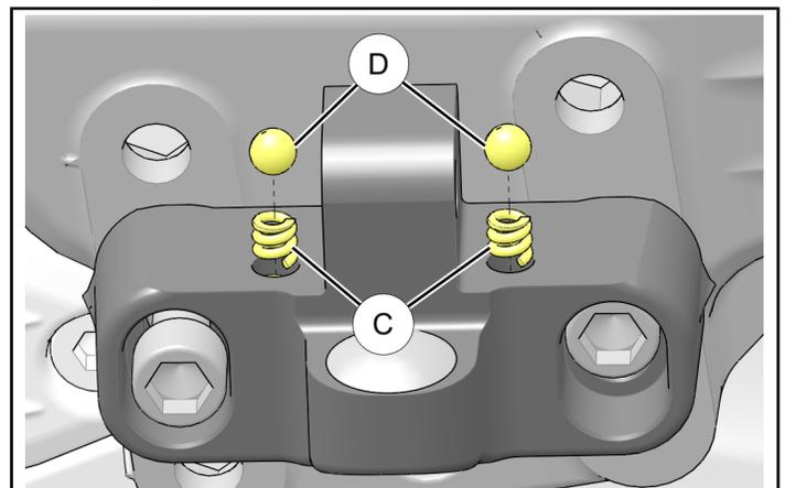
6. Carefully place Floorboard ① into position, depressing springs and balls into pivot. Align holes and insert pin ② from front side.
