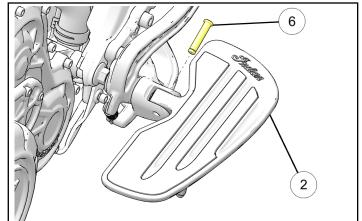
8. Install retaining ring 7 onto pivot pin 6.
