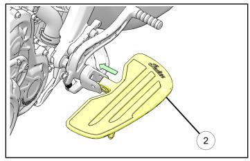
7. Install pivot pin 6 through mount and floorboard 2.
