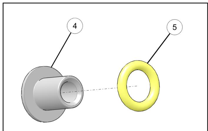
5. Install the floorboard bushing sub-assembly ④ ⑤ into left ① and right ② floorboards.
