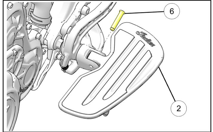
6. Slide RH floorboard ② into mounting slot.
