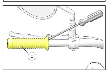
3. Firmly grasp left grip © and remove it from handlebar.
