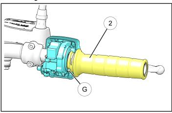
2. Reinstall back side of switch housing (£) and four screws (D). Torque screws to specification.
