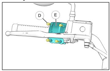
2. Separate right switch housing halves and slide right grip and throttle tube (f) off handlebar.
