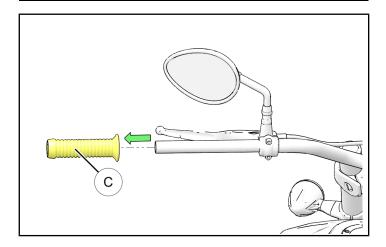
4. Remove any adhesive residue or grip material from handlebar.
