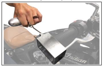
4. Keep tool centered so it does not touch hand grip. Pull on scale connected to tool eyelet.
