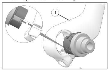
3. Install screw ① into mirror assembly ① and torque to specification.
