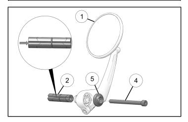
2. Assemble opposite side mirror, ensuring that friction ring, mounting spool, split nut, and end cap are assembled in opposite direction.
