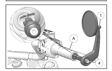
2. Adjust mirror to desired position and torque screw (4) to specification.
