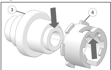
2. Assemble friction ring and mounting spool into mirror assembly ①. Align slot in mirror assembly with slot in friction ring.
