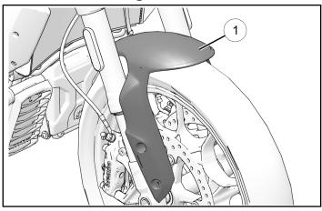
2. Loosely install fender ① with four mud guard fasteners ② and four washers ③, before torquing hardware.
