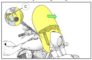
2. Lift windshield/wind-deflector straight up off lower bushings and off motorcycle.
