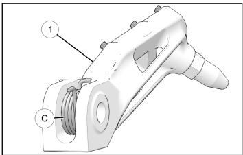
3. Place foot peg ① into foot peg mount and pass retained pin ⑧ through mount and foot peg ①. Ensure spring-end ⓒ is fitted in foot peg mount cavity.
