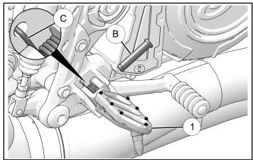
4. Secure pin ® with retaining ring 4.
