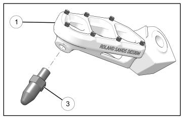
2. Set retained foot peg spring © within foot peg cavity ①. Ensure two spring-ends are oriented as shown.
