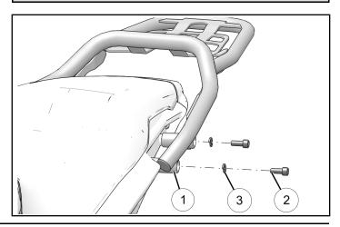
3. Install RH side of luggage rack with two fasteners ② and two washers ③.
