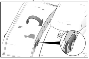
5. Ensure bushings are fully seated within spools before closing quick release latches ③.
