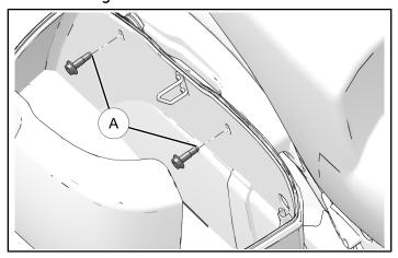
3. Tilt saddlebag away from frame and remove from vehicle.
