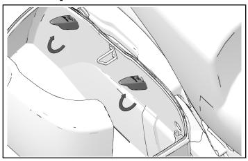
6. Tilt saddlebag away from frame and remove from vehicle.
