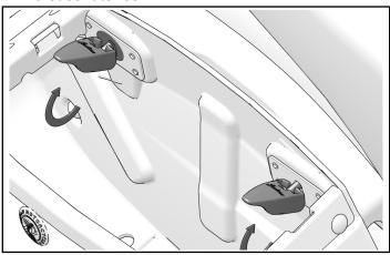
2. Lift saddlebag mounts off quick release spools and tilt away to remove from motorcycle.
