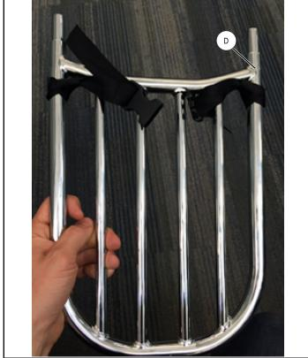
2. Install the correct mounting plate for your application. For the trunk rack, install the mounting plate with the wide clip (E). For the luggage rack or solo rack, install the mounting plate with the narrow clip ②. Slide the correct plate into the sleeve on the bottom of the bag, and secure the two snaps between the bag and the plate (F).
