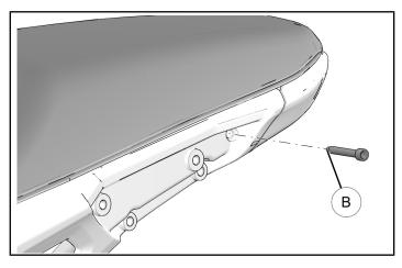
5. Reinstall two passenger handles with two screwsA per handle.
