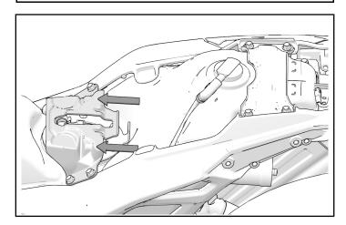
3. Slide accessory seat into seat support bracket and into front mounting bracket.
