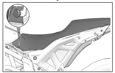
4. Secure rear of accessory seat with two retained screws (B).
