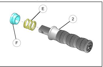
4. Slide the right-hand passenger peg (2) into the peg slot by compressing the spring. Compress the spring until pivot pin holes in the mount and peg are aligned.
