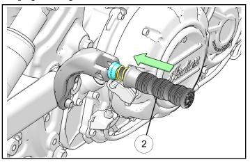
5. Install the pivot pin (B) through the peg mount and passenger peg (2).
