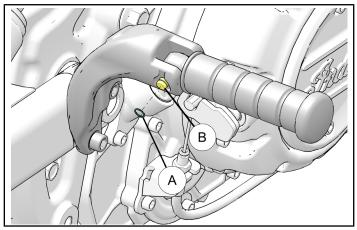
2. Remove the pivot pin (B) from the right-hand peg mount and remove the peg (D) with plastic washer (C).
