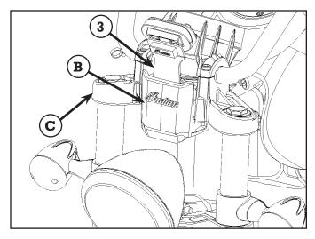
6. Fasten wire cover and phone mount to vehicle using two M6X16 fasteners (7) provided in kit. Torque to 84±8 in-lbs. (9.24±0.88 Nm). See figure.
