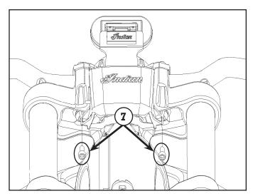
7. Cycle handlebars to full left and right stops and verify no pinching or binding of components is present. Adjust if necessary.
