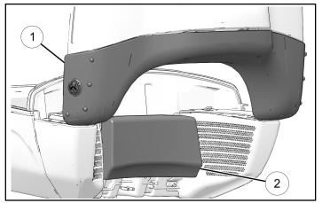
4. Install nine screws ③ to secure pads to trunk. Install two screws ③ with reserved washers ④ and cable eyes. Torque to specification.
