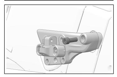
3. Adjust pivot mount to desired position and tighten two pivot mount fasteners ①.
