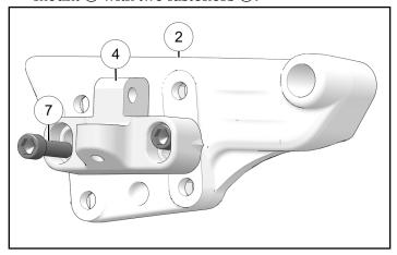
2. Install mount assembly with one retained fastener.
