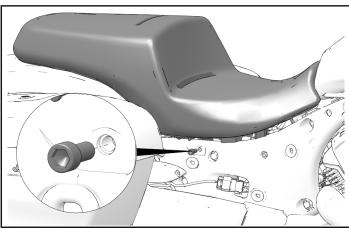
Pull seat rearward, then upward to disengage seat from frame mount and hat bushing. Do not allow seat mount brackets to contact rear fender.
