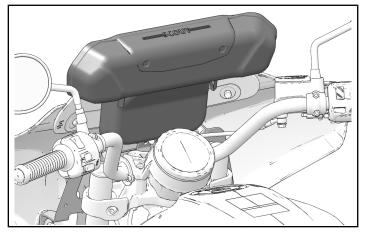
2. Attach bag with hook and loop straps around fairing bracket as shown.
