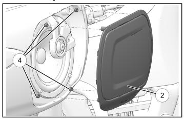
7. While applying light pressure to hold grill ② in place, install speaker cover ④ (from Kit PN 2883670-XXX) and four screws ③ (from Speaker Grill Kit PN 2883669). Ensure wiring harness is routed through opening in cover as shown. Torque screws to specification.
