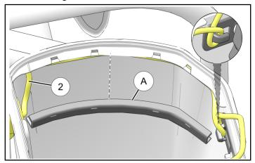
3. On underside of saddlebag lid, insert wire harness ② into Wire Cover ⑥ and adhere wire cover to underside of saddlebag lid as shown.
