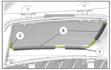
2. Carefully remove wire channel cover (A) from front upper edge of saddlebag. Route saddlebag harness (2) through hook as shown and along channel and reinstall cover (A).
