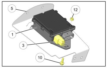
5. Connect Smart Power Supply Harness connector **2E** (from LH Saddlebag/Smart Power Supply Harness ②) to Smart Power Supply Module ①.
