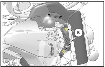
5. Pull nacelle and headlight assembly © from bike, disconnect headlight electrical connector D. Carefully set assembly aside.
