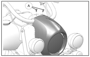
3. Turn handlebars to right until locked. Remove and retain two screws and washers <sup>®</sup> from inside of nacelle.
