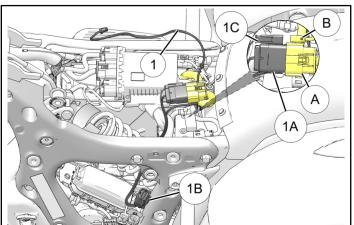
Route wiring and connector 1D around ECU along frame and out opening in right side frame as shown.
