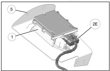
6. Install power supply mount ⑤ into LH saddlebag. Ensure LH Saddlebag harness ② is routed through opening in lower corner of mount as shown. Secure mount with two new screws ⑨ and two push pin rivets ⑪. Torque new screws ⑨ to specification.
