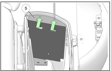
3. Carefully drill two 5/16 inch (8 mm) holes in marked location.
