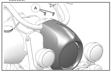
5. Ensure all wires and cables are properly tucked inside nacelle. Ensure nacelle is properly aligned and torque screws to specification.
