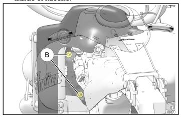
4. Turn handlebars to left until locked. Remove and retain two more screws and washers (B) from inside of nacelle.
