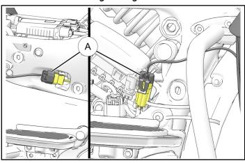
Open saddlebag lids, unplug saddlebag lock wire connector ®, remove and retain two hex head screws © from saddlebag lock assembly ®. Remove wiring from channel E.
