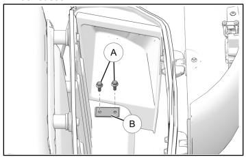
2. Using power supply mount (5) as a template, set in place and mark location of two holes.
