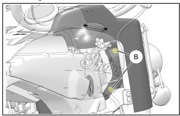
3. Turn handlebars to right until locked. Loosely install two retained screws and washers (B). **DO NOT tighten screws at this time.**
