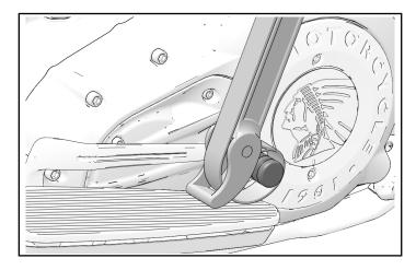
2. Align accessory peg ① with heel shifter and install with peg fastener ②.
