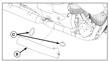
3. Cut through band clamps (C) of two remaining heat shields (D) and (E) and slide them down the exhaust pipe away from the engine to remove as shown in figure.
