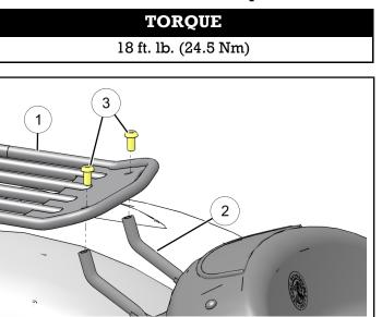
IMPORTANT Re-torque fasteners after 500 miles (800 km) of riding.
