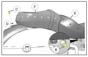
c. Lift and slide attached driver E and (if **applicable**) passenger F seats backwards.
