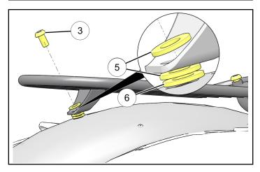
c. Torque two screws ③, connecting luggage rack ① to rack mount ②, to specification.
