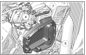
4. Rotate clamp ① so screw © is behind airbox and out of view. Torque clamp screw to specification.
