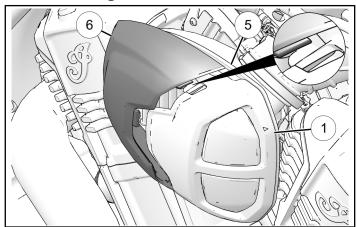
11. Secure airbox rear cover 6 with one bolt 11 as shown. Torque bolt to specification.
