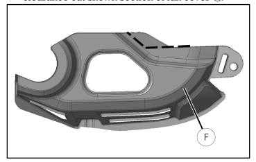
10. Using screw ① included in 2884117 kit ② and retained screw ④, install new canister bracket ③ on LH side as shown.
