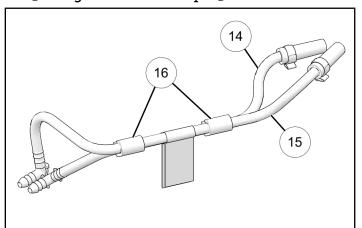
7. Route preformed vent lines under and to left of LH cover bracket ① and through engine v-gap.
