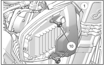
10. Slide airbox rear cover 6 onto airbox base 5. Ensure hooks from rear cover are inserted into front cover 1 as shown.
