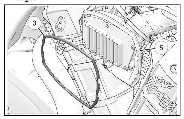
8. Install airbox front cover ① by sliding cover from back to front at an angle. Insert cover tabs into hooks on plastic base ③ as shown. Rotate back of cover onto airbox.
