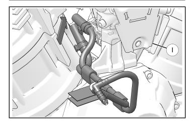
8. Locate OEM purge vent line connection © and OEM tank vent line ® on RH side of vehicle. Ensure vent line assembly is routed as shown. Connect vent line ® to tank vent line connection and vent line ® to purge vent line connection.
