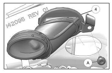
3. Connect airbox base 5 to duct 4 using clamp 7. DO NOT tighten clamp at this time.
