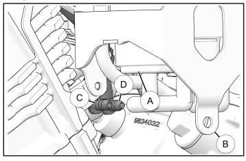
2. Lubricate canister band (E) with Isopropyl Alcohol to avoid damage to band. Remove and retain canister (A) from bracket (B). Discard bracket.
