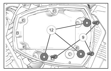
6. Install filter with four, pre-inserted screws ①. Torque screws to specification.
