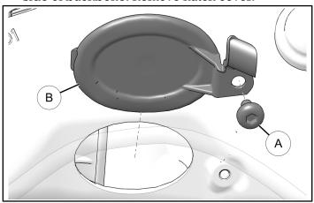
2. Install new airbox duct 4 to backbone using retained screw A. Torque screw to specification.
