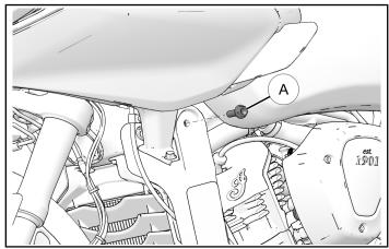
2. Install LH highway bar ① using retained bolt ⓐ and one new bolt ④ as shown. Torque bolts to specification.
