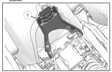
3. Route any surrounding wire harnesses in front of backrest mount ① as to not allow wires to sit over or on top of mount. Route fuel line through cable tie clip ③ and secure to mount as shown.
