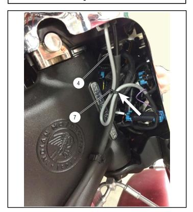
10. An accessory phone mount is strongly recommended. If Accessory Nacelle Mount (Kit PN 2880930) is installed, route 3.5 mm jack 3 through key hole on Nacelle Accessory Mount bracket 2.
