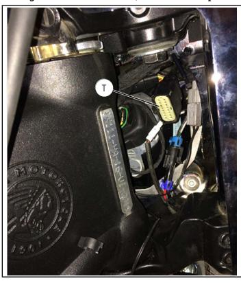
2. Attempt to locate un-used power connector ①, without opening headlight housing, by turning handlebars to one side. Connector will be tucked into headlight housing. See figure. If 16-pin connector and power connector are both accessible, skip to Step 8. Otherwise, access can be gained in Steps 3-7.
