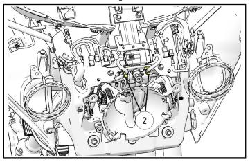
8. Place the upper dash back in place, if it was removed completely, making sure the windshield linkage arms are in their designated cutouts in the upper dash.  Reinstall Allen head M5 screw (K), metal top hat, rubber washer and plastic washer at each side of the windshield support bracket and two M4 screws (J) to dash storage removed in Step 2. Torque screws to specification.
