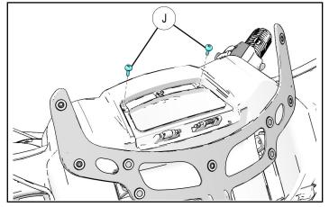
10. Reinstall two Allen head M4 screws (H) removed in Step 1. Torque to screws to specification.
