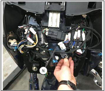
6. Locate the 4-channel amplifier ① from this kit. Plug in the 16-pin connector that was removed from the old amplifier, and slide the new amplifier under the cast faring support in the same orientation. The plug for the harness should face the right side of the motorcycle. Fasten the amplifier ① with the retained three bolts (M), removed in Step 5. Torque fasteners to specification.
