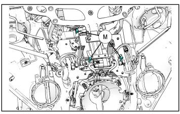
5. Separate the wires and slide the amplifier (N) out from its position behind the cast faring support. Once accessible, disconnect the 16-pin connector on the amplifier.
