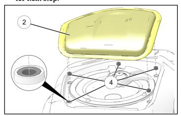
6. While applying light pressure to hold grill ② in place install five screws ③ (from *Speaker Grill Kit PN 2883665*). Torque screws to specification.
