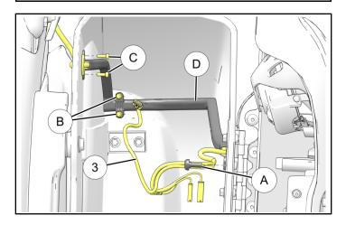
4. Route saddlebag harness wire through built-in channel in lid (shown with arrow). Plug the following terminals in:
