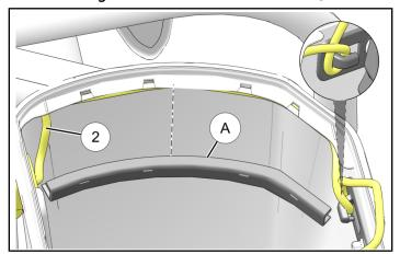
2. On underside of saddlebag lid, insert wire harness ② into Wire Cover ⑤ and adhere wire cover to underside of saddlebag lid as shown.
