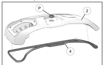
2. Hold new lid ②vertically and install to saddlebag hinge using four retained screws (M). Torque screws to specification.
