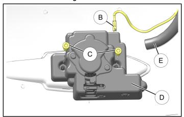
3. Remove saddlebag lock assembly ①, handle ⑤ and lock cylinder grommet ⑥, and set aside. Remove two screws ⑥ from lid hinges and remove lid. Repeat for second saddlebag lid.
