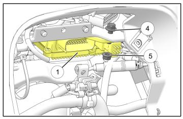
5. Locate connector for Power Supply Module ① and plug connector into module, press on connector until an audible "click" is heard. Gently pull on connector to ensure connector is fully seated.
