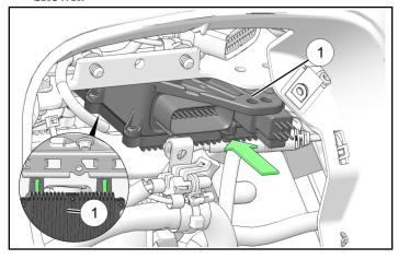
4. Secure Power Supply Module ① with new bolt ④ and nut ⑤. Torque to specification.
