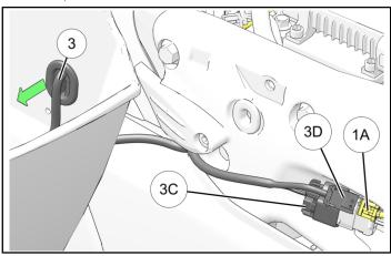
2. Repeat step one for LH wire harness ② connecting LH Chassis Connector (2B) into underseat harness ① LH Saddlebag Audio Harness Connector (1B).
