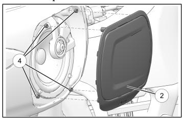
7. While applying light pressure to hold grill ② in place, install speaker cover ④ (from Kit PN 2883670-XXX) and four screws ③ (from Speaker Grill Kit PN 2883669). Ensure wiring harness is routed through opening in cover as shown. Torque screws to specification.
