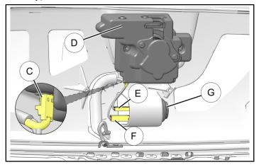
3. Remove and retain two screws (H) and remove lock assembly (D) and handle (J) from lid. Remove 12V outlet (G) from lid. (12V outlet in RH Saddlebag only.)
