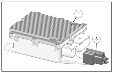
3. Install Power Supply Module ① into fairing bracket. Ensure two tabs slide into bracket as shown.
