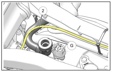
8. Route wiring (2) under upper frame (H). Secure wire to main harness with cable tie (4).
