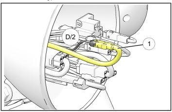
2. Reconnect wiring in headlight assembly and reassemble headlight. Torque headlight retaining ring screw to specification.
