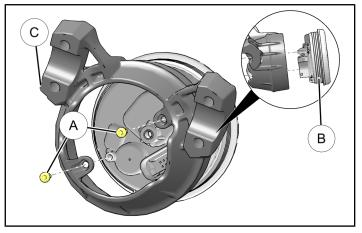
Insert speedometer (B) into new speedometer mount (3) and secure with two retained screws. Torque screws to specification.
