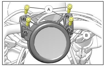
Carefully lift speedometer mount from bike until rear connector C can be accessed. Unplug connector C and remove speedometer mount B.
