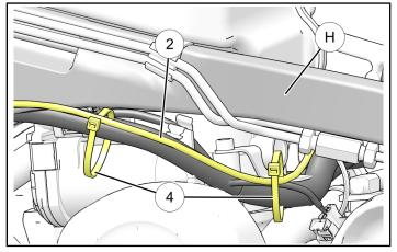
Route wiring (2) behind frame(H) and secure to existing harness (K) with new cable tie (4). Continue to route wire (2) behind fork (1) toward headlight housing.
