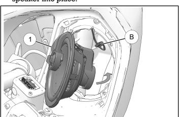
Rotate speaker so tweeter is located in top inner corner of opening as shown. (RH Speaker shown.) Secure with retained screws (A). Torque screws to specification.
