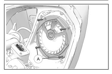
2. Rotate speaker assembly and remove. Unplug speaker connector (8).
