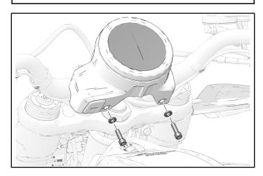
2. Disconnect all electrical connections before removing instrument cluster from handlebar.
