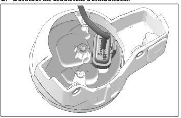
3. Install instrument cluster with two retained fasteners and two retained washers.
