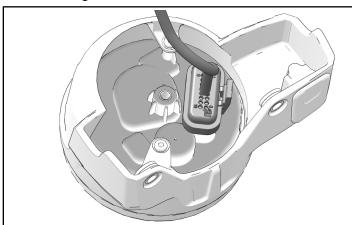
3. Keep two bushings and two rubber washers from rear of instrument cluster.
