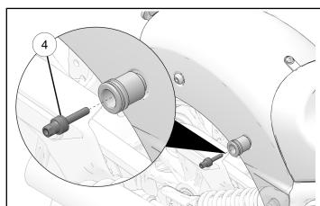
4. Keep rubber bushing ② and accessory mounting screw ⑤ for installation of accessory saddlebags.
