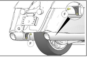
2. Slide slot of bumper brackets (2) and (3) between exhaust brackets (6) and exhaust frame at lower fastener location. Line up top fastener locations of exhaust bracket (6) and bumper bracket (2) to install two fasteners (F) retained from **Previous Step**.
