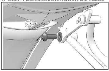
2. Install right-hand number plate with one front fastener 8 and one rear fastener 1 and nut 1.
