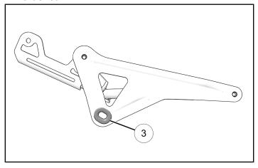
3. Install accessory mount to weld bracket with fasteners ①8 and nuts 101.
