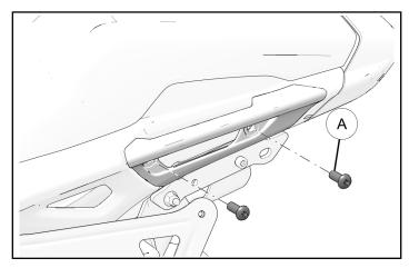
5. Install left hand number plate 5 onto weld bracket at grommet location and install at top mounting location with two number plate fasteners 9.
