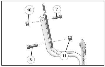
3. Install accessory mount to sub-frame with two accessory mount fasteners, included in *Accessory Mounting Kit P/N 2883842*
