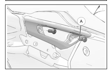
3. Install right hand number plate ④ onto weld bracket at grommet location and install at top mounting location with two number plate fasteners ⑨.
