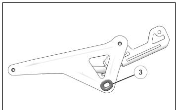
2. Install accessory mount to weld bracket with fasteners  $\Im(8)$  and nuts  $\Im(1)$ .
