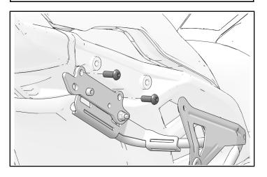
2. Install passenger handle with two retained handle fasteners (A).
