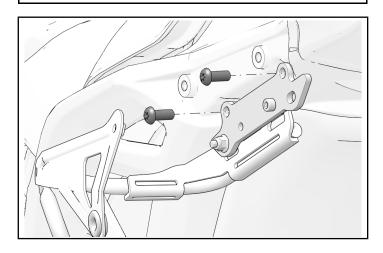
4. Install passenger handle with two retained handle fasteners (A).
