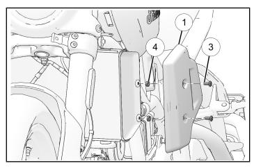
2. Install RH radiator guard ② with two radiator guard fasteners ③ and two spacers ④.
