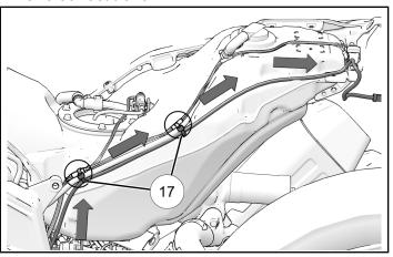
4. Let license plate chassis harness hang over right-hand side of vehicle during left-hand subframe reinstallation.
