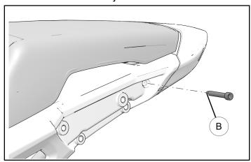
3. Slide seat back-and-up, to ensure seat slides out of mounts, to remove from motorcycle.
