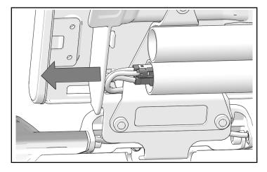
3. Remove and retain three screws (A) to remove license plate / rear fender assembly from mounting arm. Carefully set mounting arm aside.
