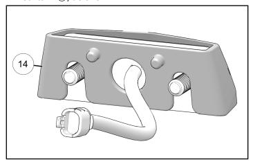
4. Install license plate light and curtain onto license plate bracket with two nuts <sup>(1)</sup>.
