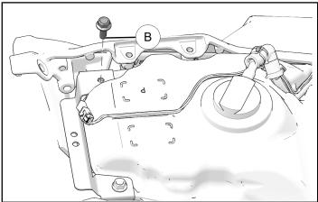
3. Remove and retain two screws © and two screws © from left-hand sub-frame.
