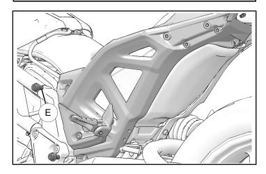
2. Install rear-end of sub-frame with two upper screws © and two lower screws ®.
