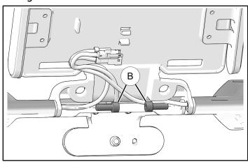
6. Remove two nuts © to remove license plate light from bracket. Route license plate light cable through bracket to completely remove from bracket.
