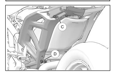
3. Torque sub-frame fasteners to specification.
