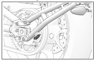
2. Cut and remove cable tie (A). Carefully pull chassis harness out of cavity and disconnect chassis harness from license plate harness.
