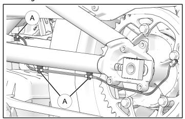
Route chassis harness along fuel line towards rear light location. Tuck chassis harness behind frame to avoid pinching when sub-frame is reinstalled.
