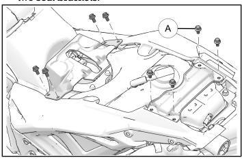
2. Remove and retain one screw ®, located between fuel tank and left-hand sub-frame.
