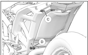
4. Remove and retain two screws (£) to remove left-hand sub-frame from motorcycle.
