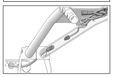
7. Place threaded rods of license plate bracket through license plate mount. Install lower bracket with two nuts ③. Install upper bracket with two screws ⑤.
