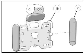
3. Route light cable through light curtain (4) and then slide retained license plate light into light curtain (4), as shown.
