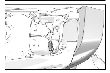
2. Remove and retain two screws (A) to remove rear light from frame.
