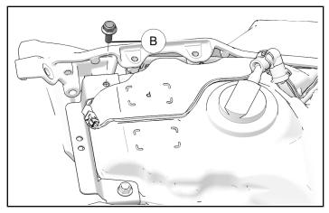
5. Install two seat brackets onto right-hand and left-hand sub-frames with eight screws (A). Torque one fuel tank screw (B) prior to torquing eight screws (A).
