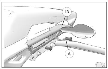
5. Route turn signal cables over license plate mount tubes, as shown.
