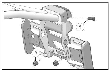
8. Secure license plate to bracket with four fasteners (5) and four nuts (9).
