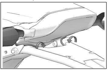
6. Join chassis harness connector to license plate light connector. Join turn signal connectors to license plate harness, installed in *License Plate Assembly* section. Secure excess cable to license plate mount with three push-pin cable ties (8).
