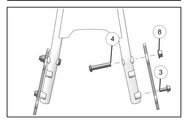
Install accessory mounting plate / license plate mount assembly onto sub-frame with two screws
