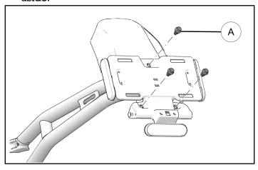
Pinch two tabs on license plate mount to disengage from debris shield. Harnesses will need to be routed out of debris shield opening during disassembly.
