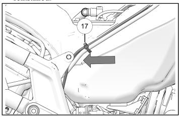
3. Secure to fuel line with two cable ties ① at circled locations.
