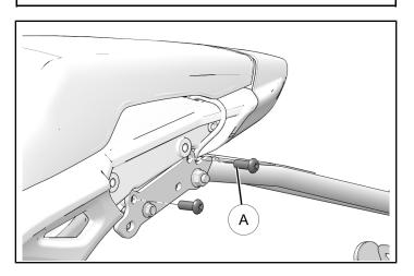
3. Install retained turn signals onto new left-hand passenger handle ③ with one screw ⑤. Ensure turn signal cable passes through passenger handle before securing with fastener.
