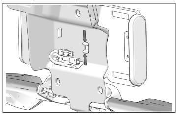
5. Remove and retain one screw ® from each turn signal.
